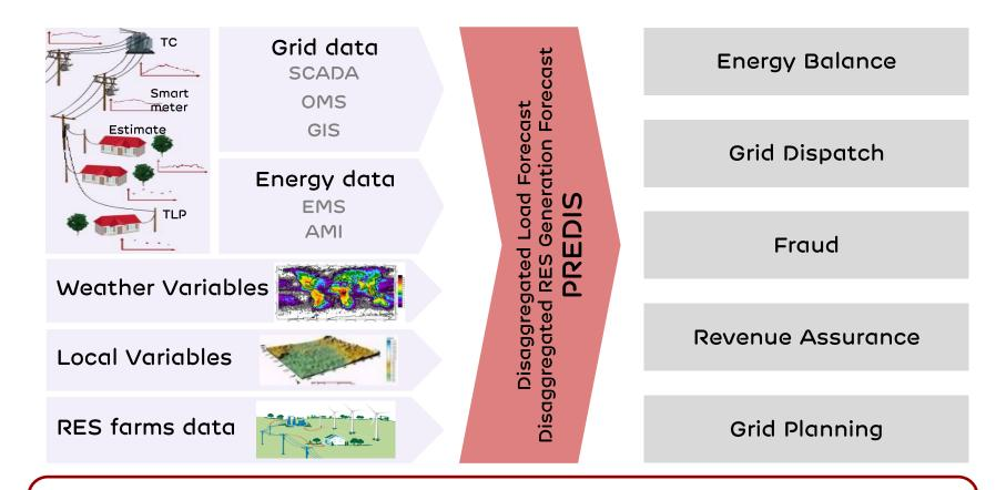
The project combines external and internal sources of data to forecast and to give results to support several operational processes
