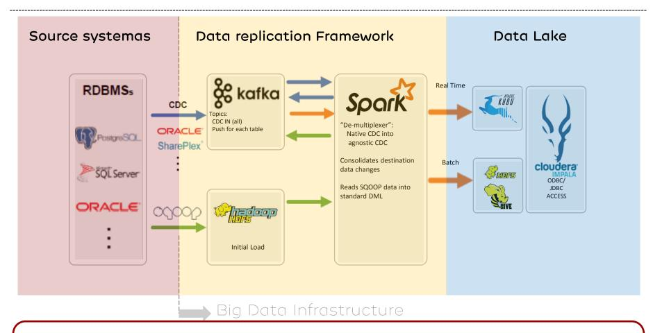
This architecture replicates the operational systems in the Big Data infrastructure, processes and consolidates the information in real time without impact to the source systems
