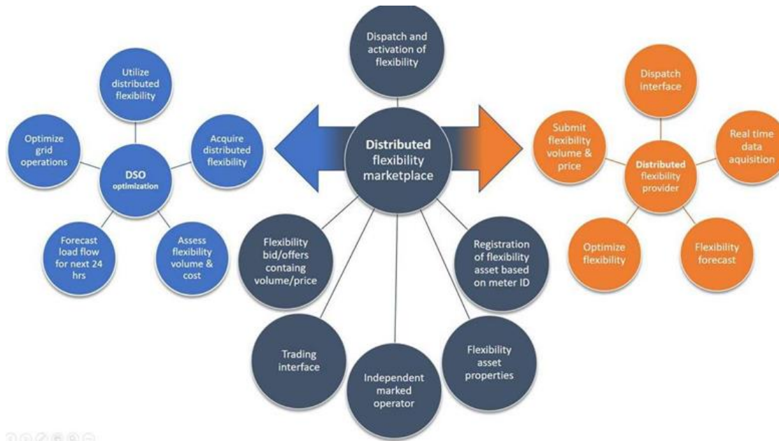
Figure 2: Example of the architecture and functionalities of the flexibility marketplace (source: Agder Energi)
